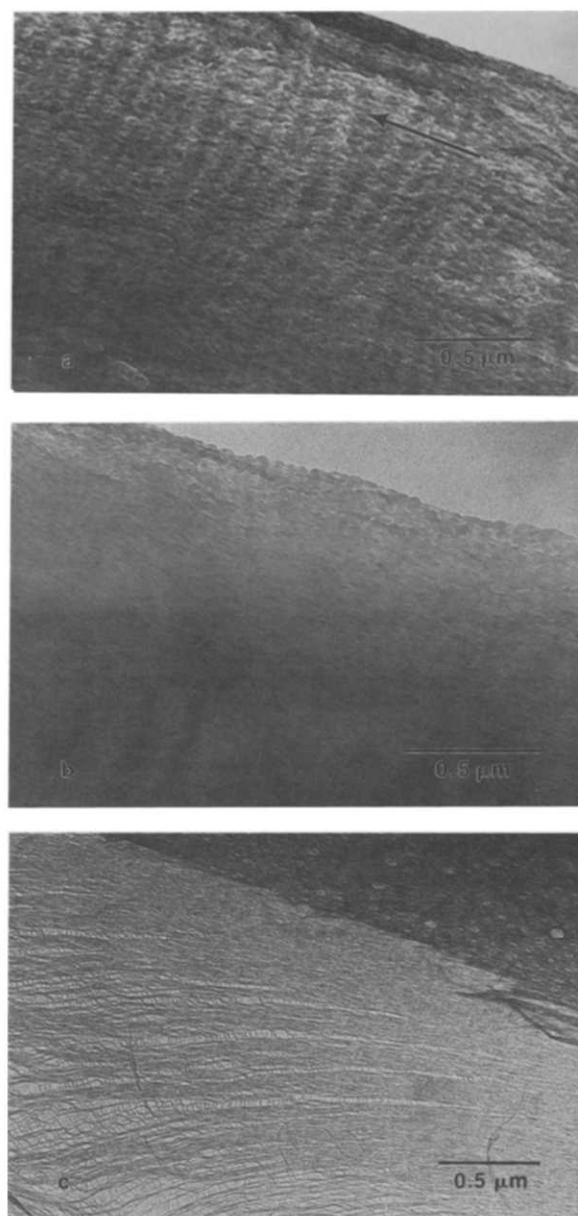
Figure 7 Electron micrograph of a methylene-chloride-quenched film after water coagulation showing the effect of quench rate on the morphology. (a), (b) 100° s -1 quench rate; (c) 500° s -1 quench rate
